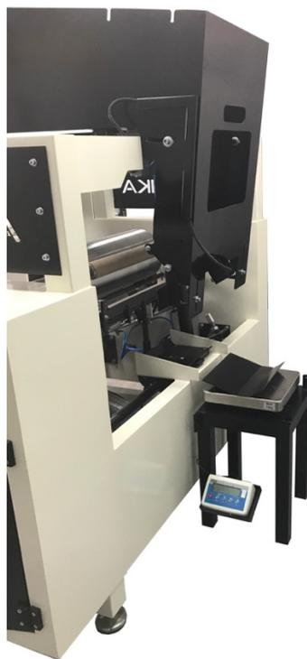
Weighing module - optional equipment of the machine.
